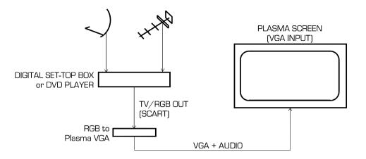
Connect the digital set-top box (or DVD player) to the RGB to Plasma VGA's SCART input, then the output directly to the plasma screen with audio. In some systems the audio may be routed to an external amplifier rather than the plasma screen.
