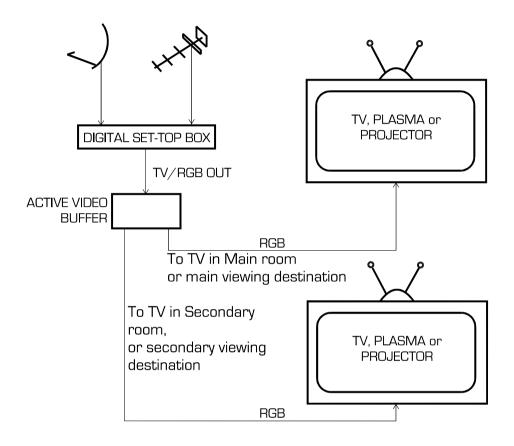
A basic configuration is to connect the digital set-top box (or DVD player) to the Active Video Buffer and then to connect two viewing devices from the Active Video Buffer's outputs. If the viewing area, for example, has a projector that is only used on occasion the Active Video Buffer allows for the projector to permantely connected as well as simultaneous viewing.
