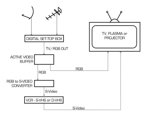
If the home-cinema system has an S-VHS or D-VHS recorder, then it would be appropriate to connect the RGB to S-Video converter to one of the Active Video Buffer's outputs. The second output of the Active Video Buffer can then deliver high quality RGB to the TV, plasma screen or projector.
